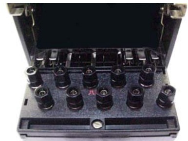
Figure 10. Separate Source Test Plug inserted in Flexitest Relay Case
